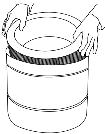
STEP 16 Replace the HEPA filter.
