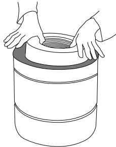
STEP 17 Replace the Carbon Canister inside the HEPA filter.
